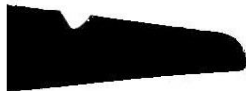
Fig. 4. Propeller Damage Type 4
