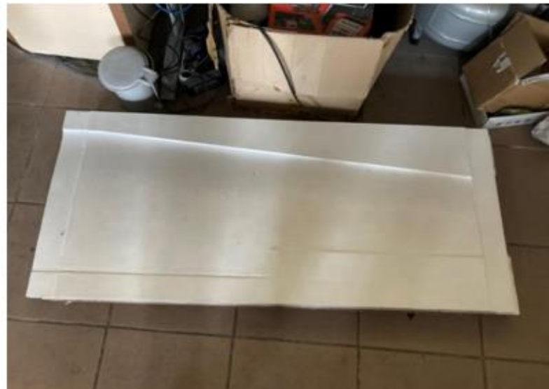
Fig. 15. MDF wood molds after CNC milling (left). After varnishing and paintwork (right)
