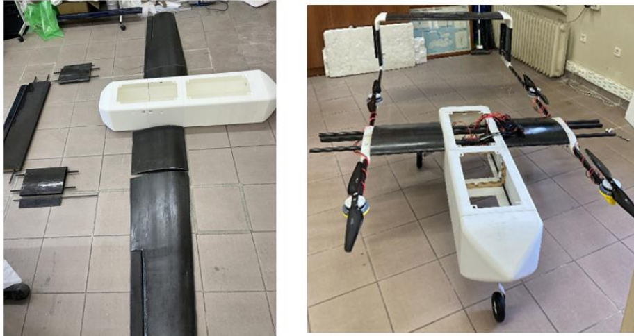
Fig. 19. The Hybrid UAV in the assembly phase (left). Partially assembled plane (right)
