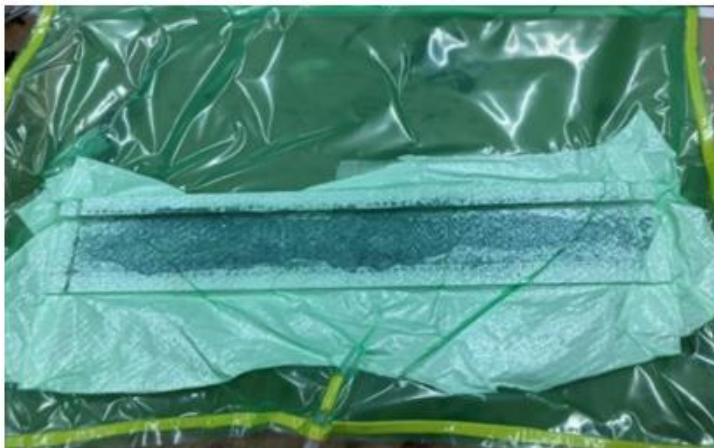
Fig. 11. Vacuum bagging process
