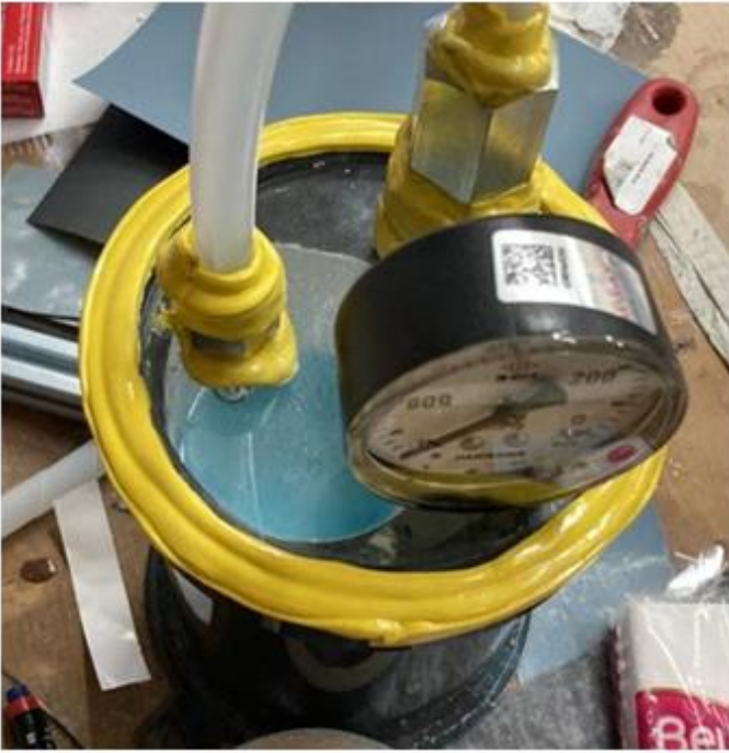
Fig. 7. Catch-pot after the process is done
