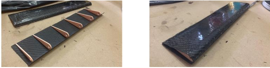
Fig. 18. The horizontal tail wing's assembly steps
