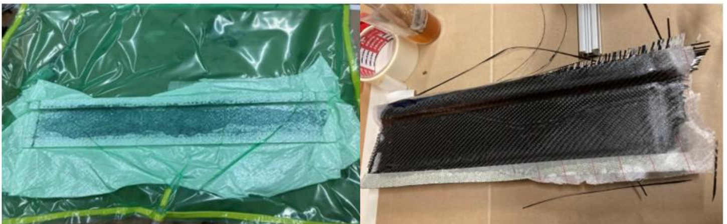
Fig. 11. Vacuum bagging process
