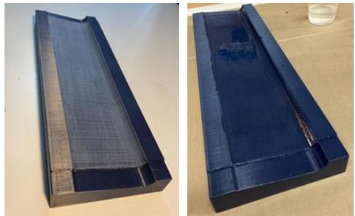
Fig. 14. Rudder mold: (a)After sanding. (b)After gelcoat
