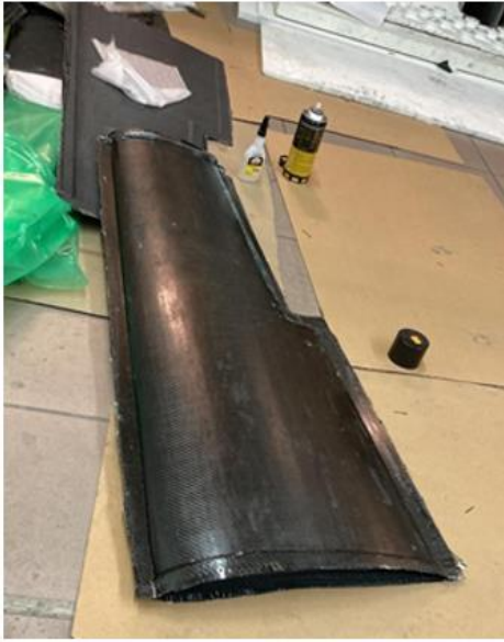
Fig. 10. A composite shell part manufactured using resin infusion technique
