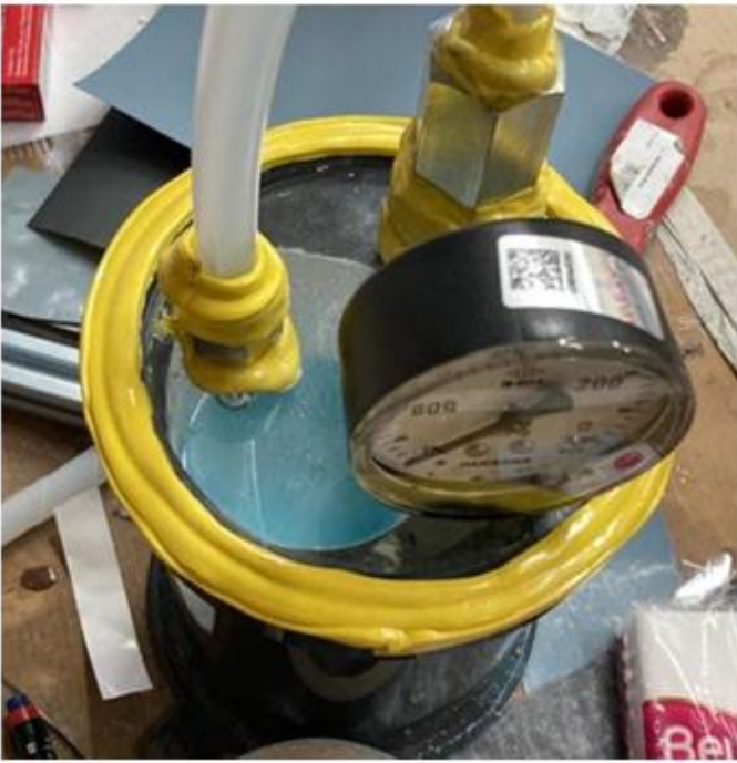
Fig. 7. Catch-pot after the process is done
