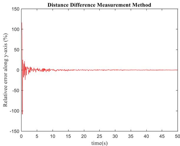
**Fig. 9.** Relative error along the y-axis when using the distance difference measurement method.
