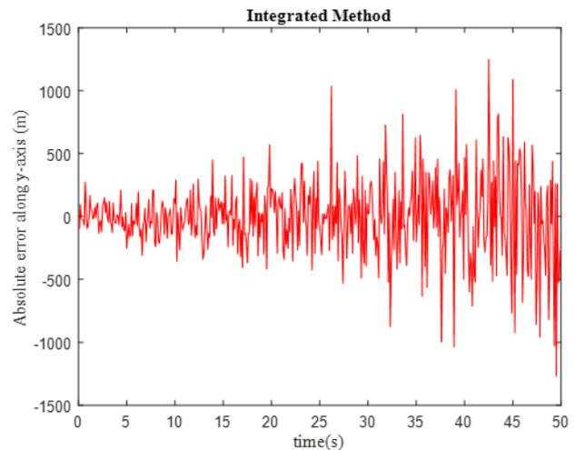
**Fig. 11.** Absolute error along the y-axis when using the integrated method.
