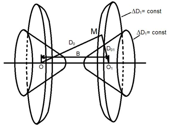
Fig.3. Illustration of the state surfaces in the distance difference measurement method.
