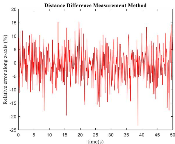
**Fig. 10.** Relative error along the z-axis when using the distance difference measurement method.
