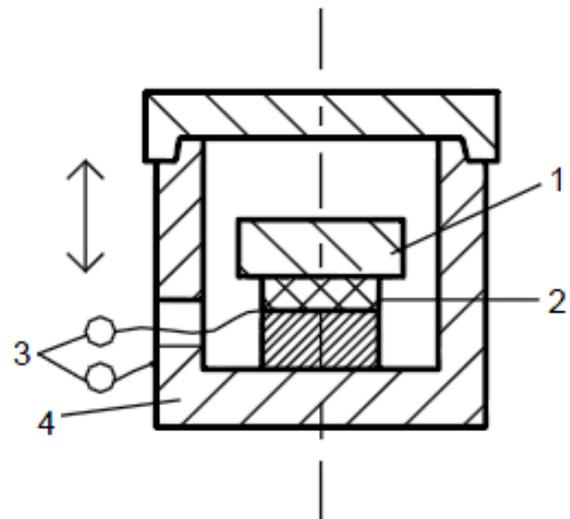
**Fig. 1.** Scheme of piezoelectric VT
