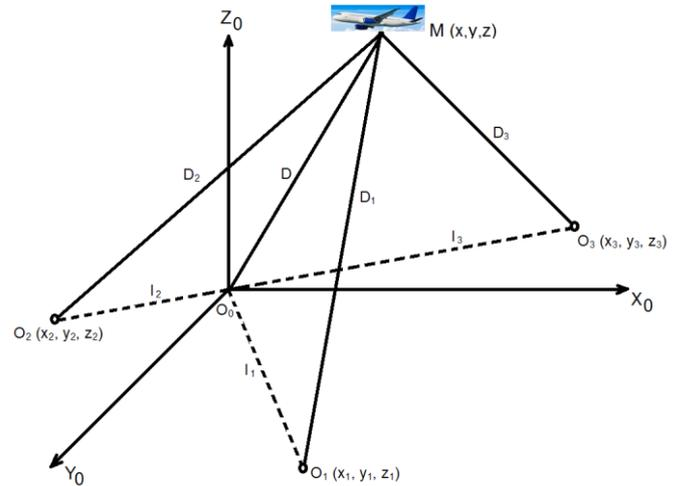
**Fig. 2.** Distance measurement method's scheme in determining the position of the aircraft
