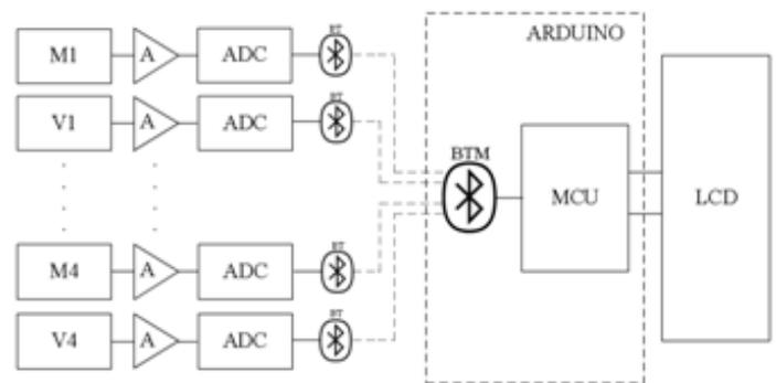
**Fig. 2.** Block diagram of the MVP system
