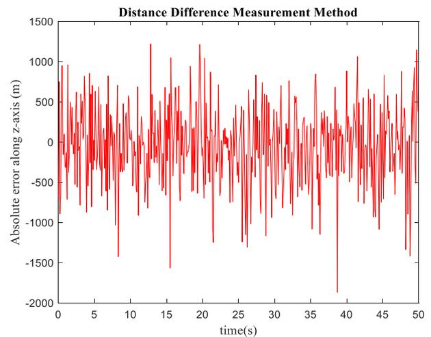
**Fig.7.** Absolute error along the z-axis when using the distance difference measurement method.
