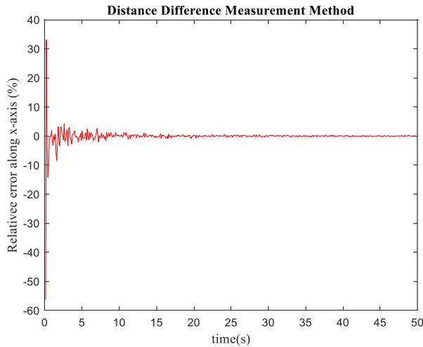
**Fig. 8.** Relative error along the x-axis when using the distance difference measurement method.
