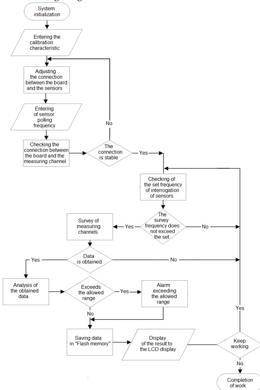
**Fig. 4.** Algorithm of measurement system operation
